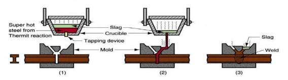
Fig: Thermit welding: (1) Thermit ignited; (2) crucible tapped, superheated metal flows into mold; (3) metal solidifies to produce weld joint.
