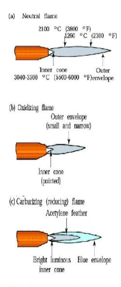
Three basic types of oxyacetylene flames used in oxyfuel-gas welding and cutting operations:
