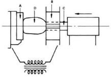
A, anvil electrode; B, gripping electrode; C, workpiece; D, upset end of workpiece
