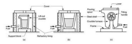
Three types: (a) lift-out crucible, (b) stationary pot, from which molten metal must be ladle (c) tilting-pot furnace
