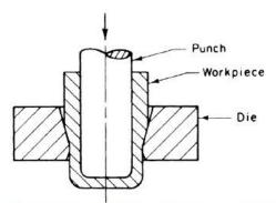
**Equipment.** Mechanical presses and hydraulic presses. **Materials.** Carbon and alloy steels, aluminum and aluminum alloys, titanium alloys. **Applications.** Shells and cups for various
