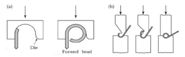
Fig .(a) Bead forming with a single die (b) Bead forming with two dies, in a press brake
