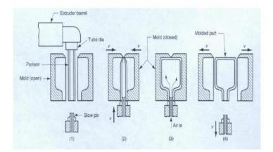
The parison can be formed by A)Extrusion process B)Injection molding process
